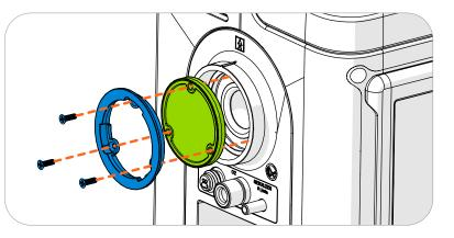
CAUTION: Do not let anything enter the cavity behind the filter during the replacement process. Do not re-install the Internal Bacterial Filter screws without using a calibrated torque driver. Foreign material inside V\*Home or using too much torque on these screws may severely damage V\*Home.
