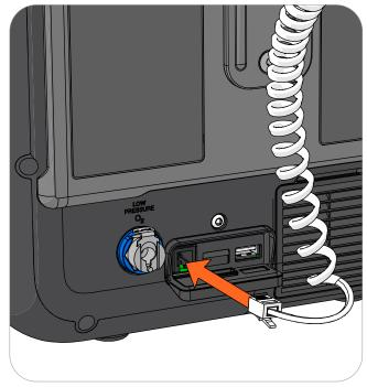
WARNING: To reduce the risk of electrical shock, ensure the Nurse Call System connected to V\*Home meets the Safety Extra Low Voltage (SELV) requirements as described in IEC 60601-1 (1988).
