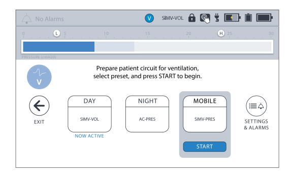
NOTE: To change Ventilation therapy settings press the Preset name and then the SETTINGS & ALARMS button. Follow the instructions described in *"Changing Ventilation Therapy Settings" on page 59* to modify Ventilation therapy settings. When configuration is complete, press < EXIT to return to the Ventilation therapy screen.
