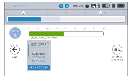
To activate and use the FiO2 monitor, it must be enabled (see *"Enabling and Disabling Prescribed Therapies" on page 72*), the Oxygen Delivery Mode control must be set to O2 Bleed In (see *"Oxygen Controls" on page 73*). When the FiO2 monitor is inactive, the High FiO2, Low FiO2, and Very Low FiO2 alarms are also inactive.
