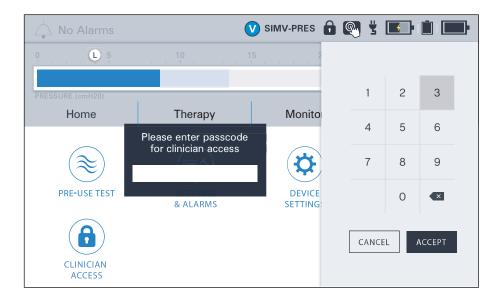
NOTE: When the Unlock Required? device setting is set to Yes, V\*Home will automatically lock after 15 minutes. To lock V\*Home manually, press the CLINICIAN ACCESS button on the Menu screen.
