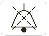
NOTE: The Internal Battery Critically Low alarm cannot be silenced until V\*Home is plugged into an external source of power. To silence the alarm after plugging in V\*Home, access the Alarm Log (by pressing the alarm banner in the upper left-hand corner of the screen or pressing LOGS in the Menu tab), and then select CLEAR LIST.
