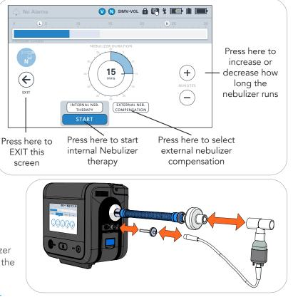
therapy or compensation will stop automatically after the set time has passed. If you want to stop the nebulizer or compensation sooner, press the STOP button.
