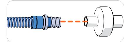
If you are using an Active Ventec One-Circuit, connect a flex tube between the circuit and the HME.
