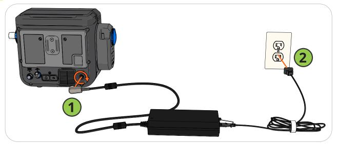
NOTE: To disconnect the power cord, twist the connector counterclockwise and then pull the connector away from VOCSN.
