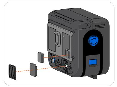
Look at the filters again to make sure they are not damaged and are clean. If they look damaged, replace them. (Replacement filters are available from Ventec Life Systems.) If the filters still look dirty, wash them again following the instructions above. If the filters are clean, dry, and not damaged, put them back in VOCSN.
