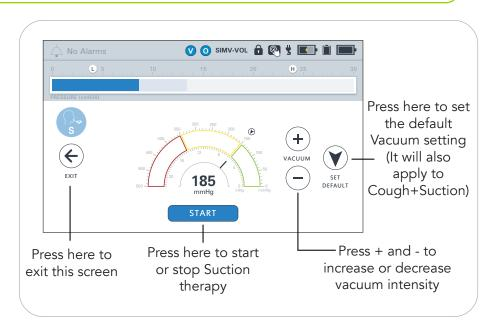
end of the suction tube, the arc should fill up all the way to the setting.
