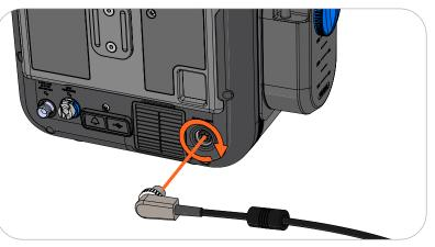
**CAUTION:** When you plug VOCSN into an external battery (like a wheelchair battery), it will pull power from it to run and charge its own batteries. This means the external battery life will be shortened. When VOCSN is connected to a wheelchair battery, the wheelchair may drive more slowly uphill.
