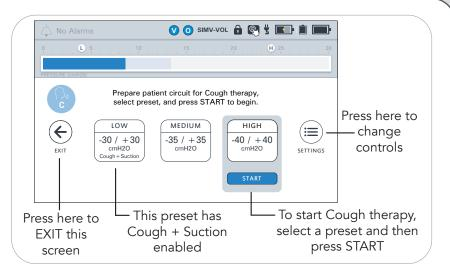
results. After Cough therapy, change back to the mask with the leak in it right away. Ventilation therapy automatically starts after Cough therapy, and continuing to use a mask without an air leak for Ventilation therapy could harm the patient.
